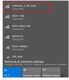
2.2 When selected "ACCESS POINT", Converter acts as an Access Point which is allowed to be connected by PC /NB /Smart Phone/ PAD. It supports DHCP server function. Soft AP broadcasts its SSID "CVIoT\_XX\_XX\_XX\_XX\_XX\_XX." PC /NB /Smart Phone/PAD should connect to this SSID and then open web browser with default IP for Converter setup.
