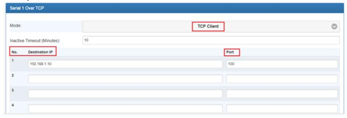
4.4 UDP: Picture as above TCP client mode. Allow to configure 4 remote destination host IP address, port number. At UDP mode, WPC-832-4 establishes a connection with remote host and sending data to remote host actively.
