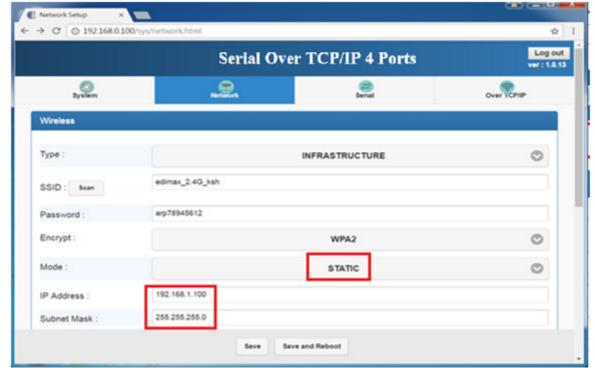
2.1.4 In NB/PC, choose same SSID to link. NB/PC must close Ethernet in advance.
